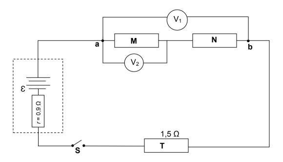
When switch  ${\bm S}$  is closed, a high-resistance voltmeter,  $V_1,$  across  ${\bm a}$  and  ${\bm b}$  reads 5 V.
